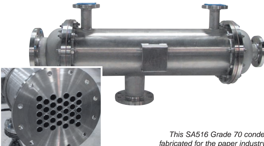
This 10" 304L stainless steel heat exchanger was manufactured for the resin production industry. It has 32 one-inch stainless steel tubes rolled into the tube sheets (see end view). It has a design pressure of 75 PSIG at 300°F.
